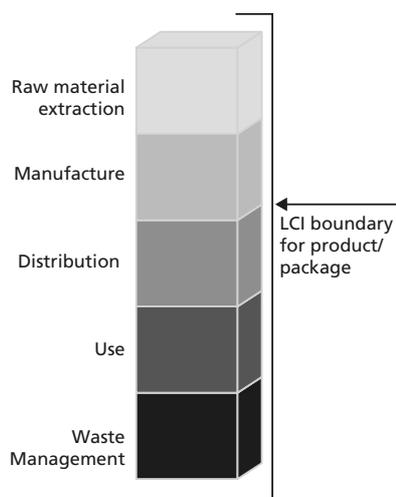
Figure 1. Boundary of the LCA for a Product or Package
